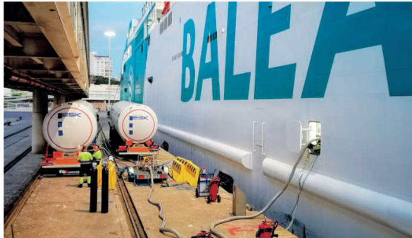
LNG bunkering operation in the port of Almeria.
